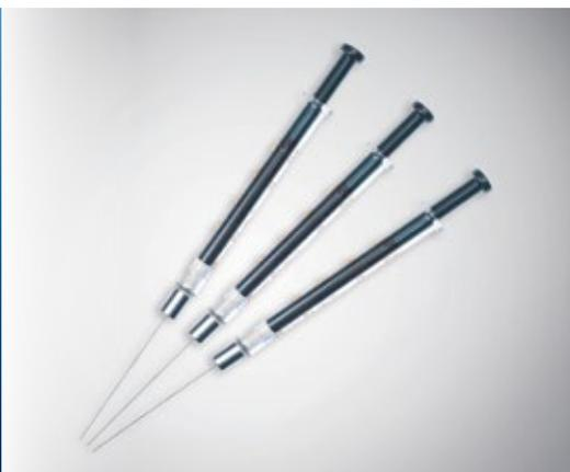
Hamilton introduces a new headspace syringe featuring a unique needle attachment in combination with the High Dynamic (HD) plunger designed specifically for PAL COMBI-*xt* Headspace Autosamplers.
