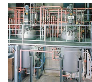
Fermentation Tanks: 2000 L Stainless Steel
