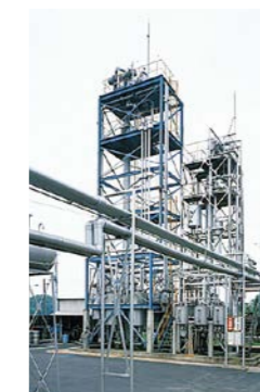
Sulzer-packed Rectification Towers: 1000 L Stainless Steel 24 plates, 2000 L Stainless Steel 36 plates
