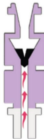
The membrane is a barrier against eluent vapours and gas leaks
