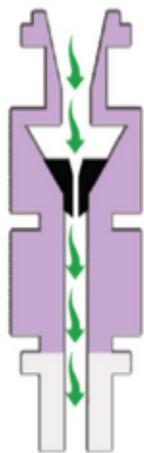
The membrane allows air to enter for pressure equalisation
